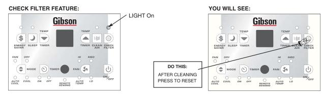
Note: This feature is a reminder to clean the Air Filter (See Care and Cleaning) for more efficient operation. The LED (light) will illuminate after 250 hours of operation. To reset after cleaning the filter, press the "Check Filter" button and the light will go off.
